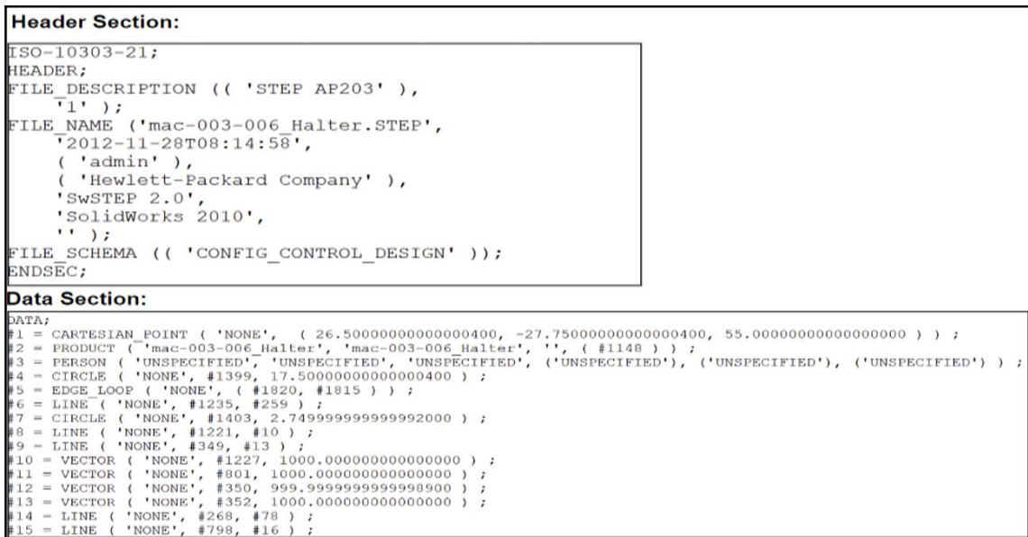
Fig 1: 3D Geometrical STEP file structure
