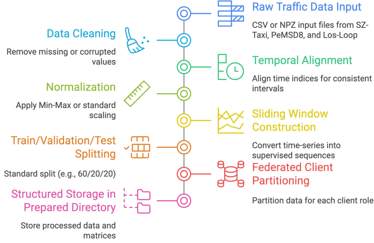
Figure 1: Data preprocessing pipeline for traffic flow prediction.
