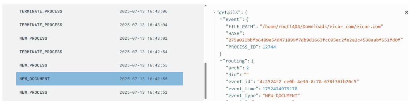
Figure 7: This log shows the event generated when the EICAR file was downloaded on the machine. This data includes timestamp and path which helps to evaluate the MTTD and MTTR. This log can be used for SOC investigations
