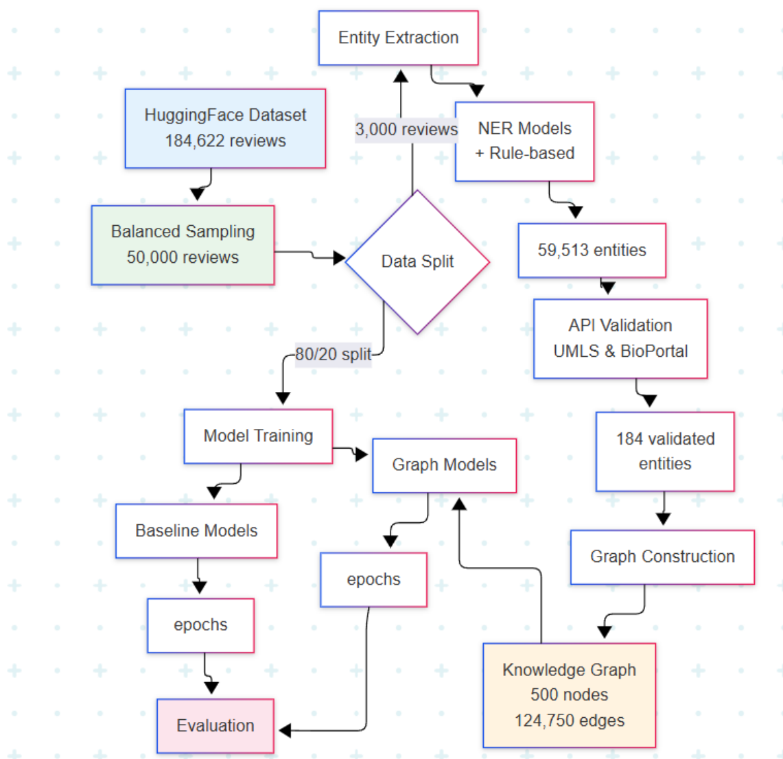
FIGURE 1 Research Methodology Workflow - illustrating the complete pipeline from data collection through model training, highlighting the parallel paths for baseline and graph-enhanced models
