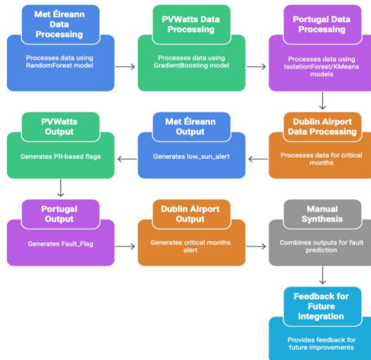
Figure 3: Fault Prediction System Architecture
