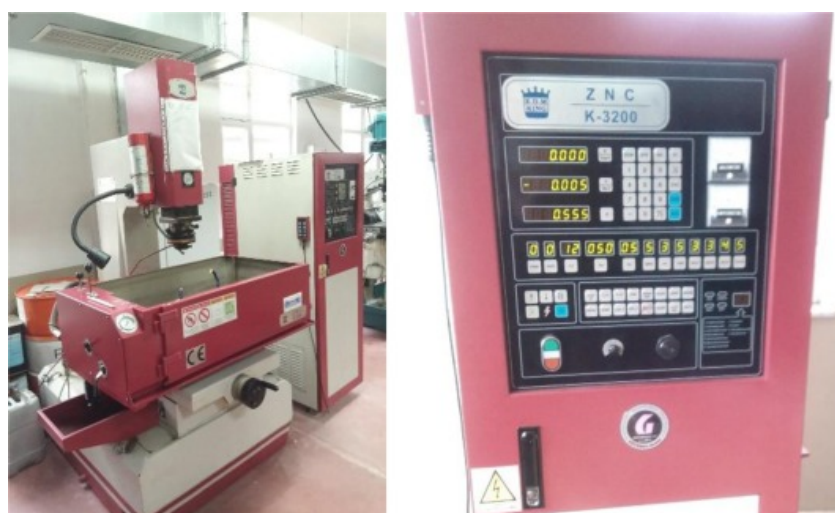
Figure 1. King ZNC K-3200 EDM machine and its control panel of the experimental setup to perform the tests [5].
