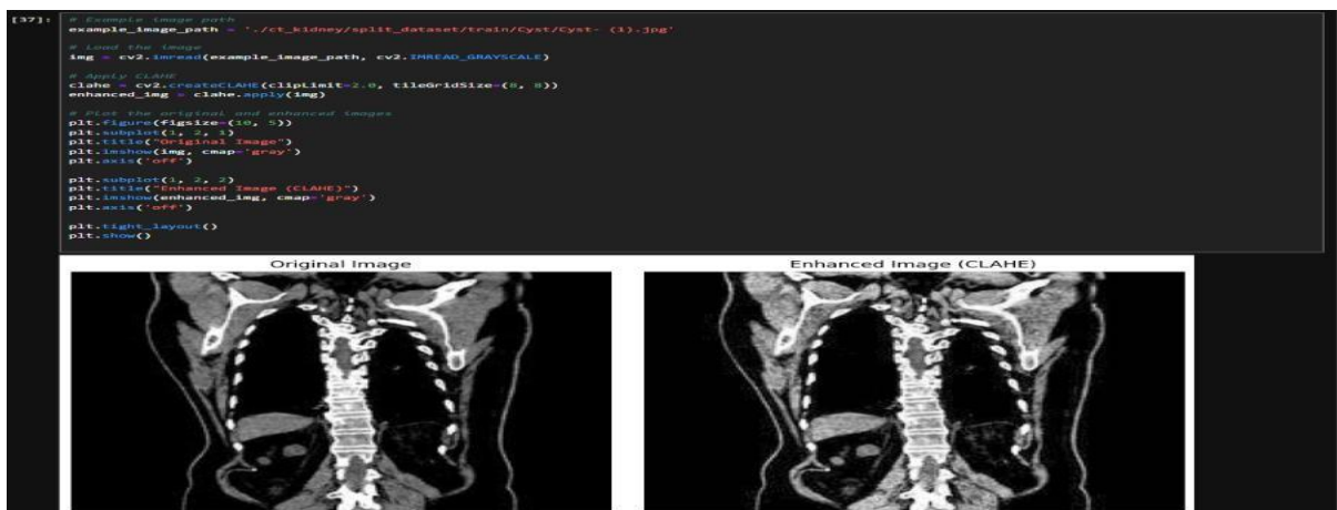
Figure 7. CLAHE has been applied to the images to improve accuracy by enhancing the contrast of the CT images
