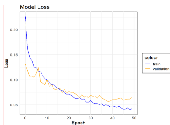
Figure 9: Loss plot for training and validation data
