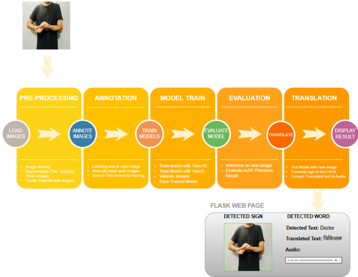
Figure 2: Proposed Methodology for ISL Recognition and Translation to text and audio
