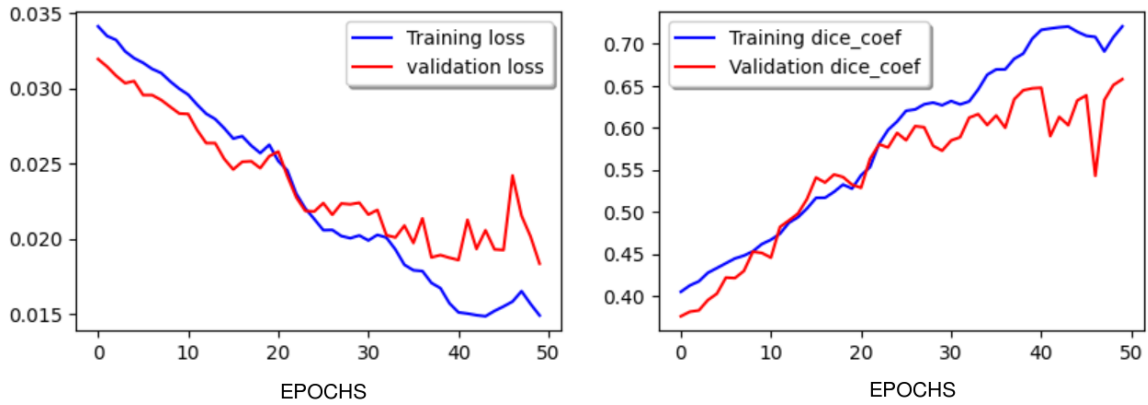
Figure 14: Unet model for 50 Epoch vs Loss and Dice Coeff. For training and validation
