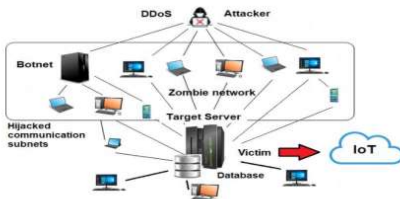
Figure 1: Flow diagram of an IoT Botnet-Driven DDoS Attack. Source of diagram: Díaz, (2020)
