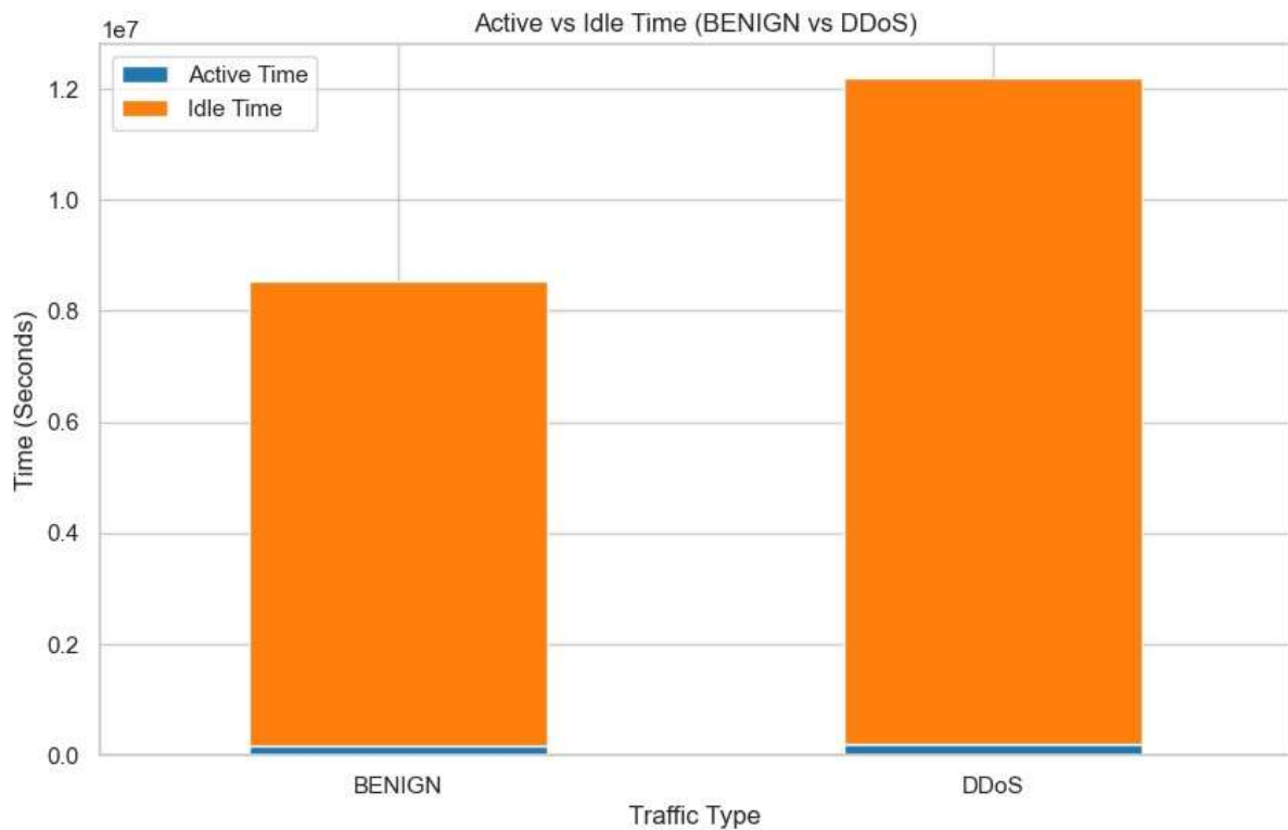
Figure 3: Proportion of "active" and "idle" times between BENIGN and DDoS traffic
