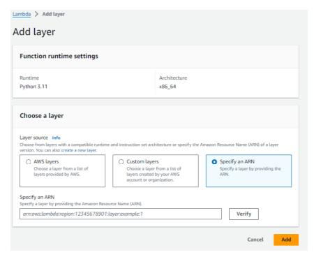
Figure 2: Adding layers in AWS lambda function
