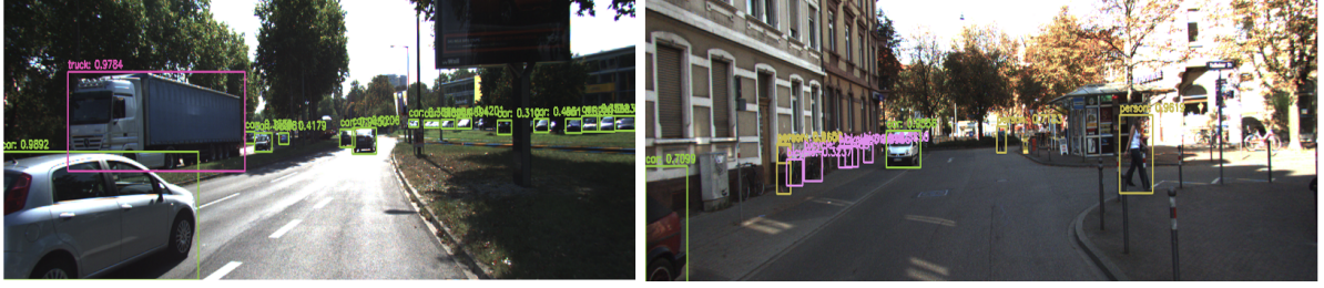
Figure 21: Ability of the model YOLOv4 to detect objects of small size and occupying small area in the image's pixel space
