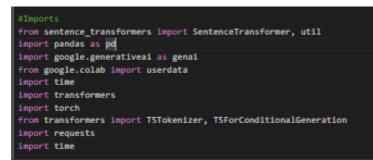
**Figure14.** The code begins by calling important libraries and modules for each of the functions included in the code. It requires the 'sentence\_transformers' library, for creating and managing sentence vectors – important for tasks like semantic likeness and other NLP processes.
