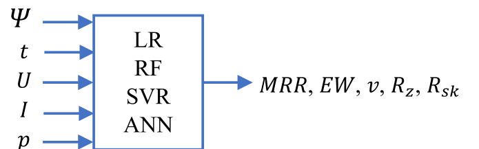
Fig. 11. Input and output parameters of the proposed prediction models for the four ML approaches.
