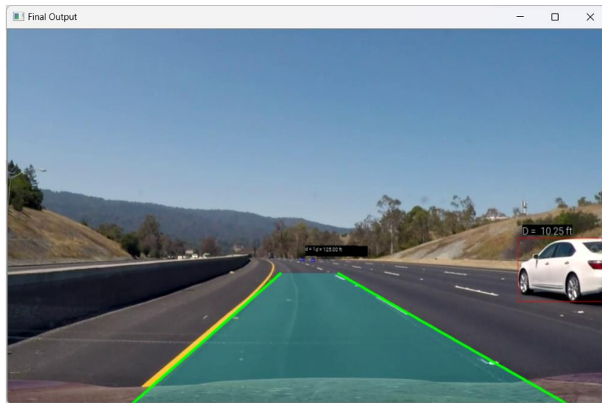
Figure 5. Lane and Vehicle Detection, Distance Estimation
