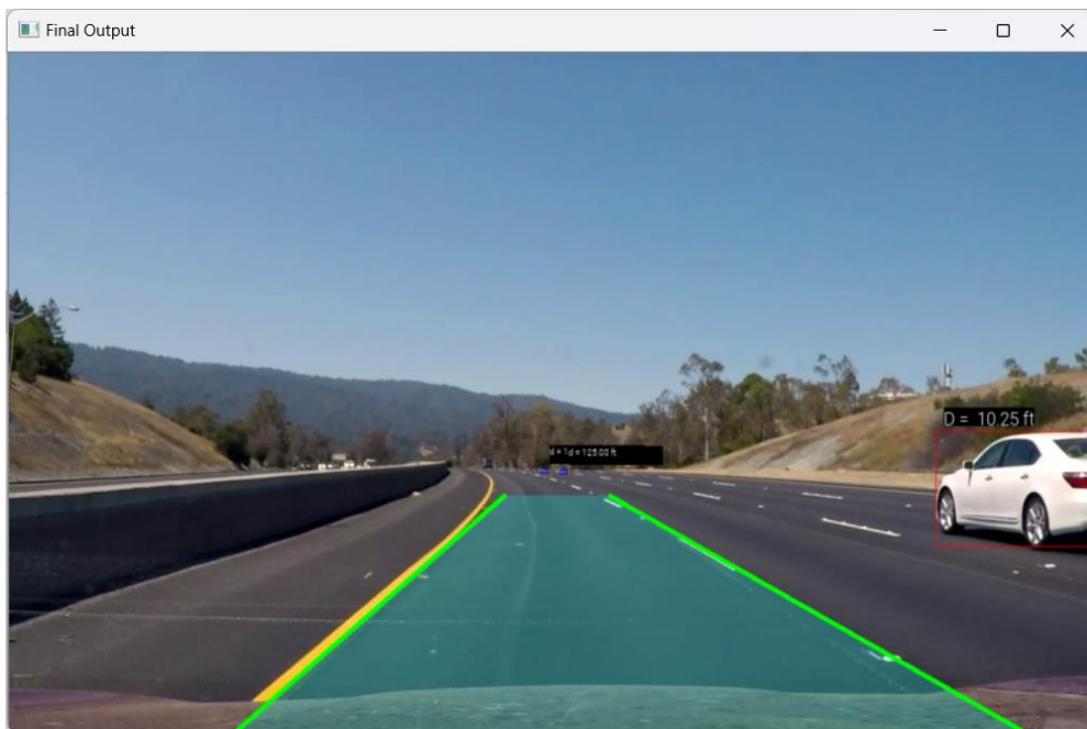
Figure 7. Lane and Vehicle Detection, Distance Estimation
