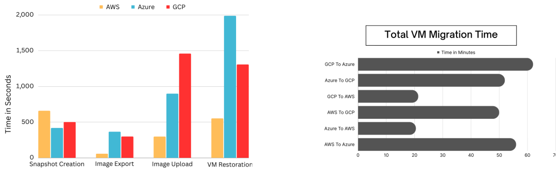
(a) Individual Process Time For Each Cloud (b) End To End VM Migration Time
