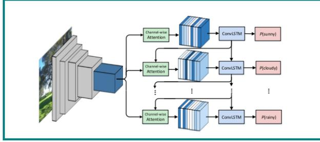
Figure 5: Proposed CNN-RNN Architecture (Zhao et al., 2018)
