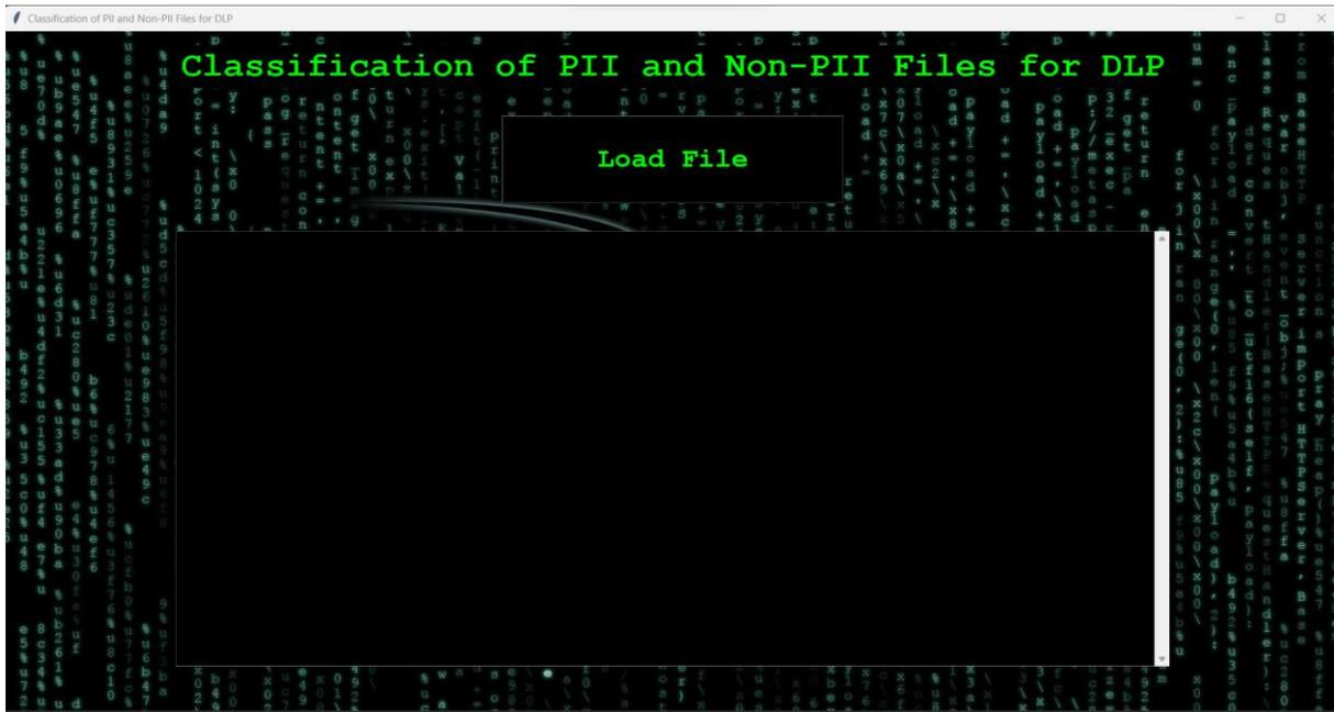
This is the basic GUI of the application now you can use the load file button to upload a text file which the application will read and then will classify the content of the file using BERT and then give alert according to the contents present in the file.
