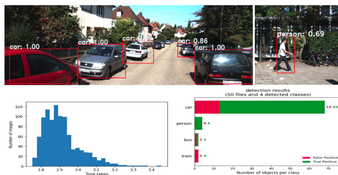
Figure 11: SSD image detection,Histogram & detection results
