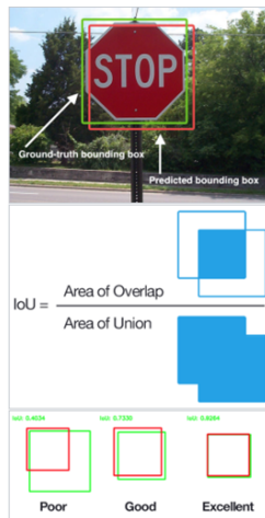
Figure 7: Extensive Calculation of the IoU
