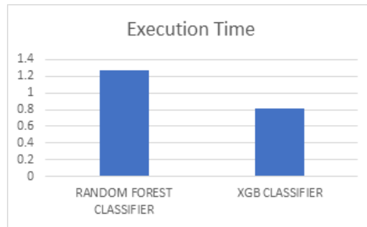
Figure 22: Execution Time comparison of Random Forest and XGBoost for Garbage Sound Detection. XGBoost is fast with a computation time less than one second i.e., with 0.81 second in comparison to Random Forest with 1.27 seconds. Hence as a conclusion, XGBoost will be deployed for canceling the garbage sound from the data.
