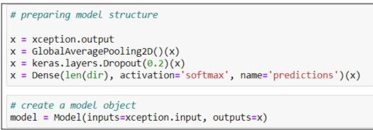
Fig.10 Preparation of Xception structure
