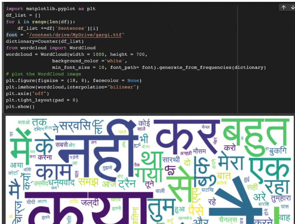
Figure 6: Upload "gargi.ttf" file which is uploaded in the code artifact. Word clouds, also known as tag clouds, are visual representations of word frequency that give terms that appear more frequently in a source text more emphasis. The word's frequency in the manuscript was indicated by how big it appeared in the image (s).
