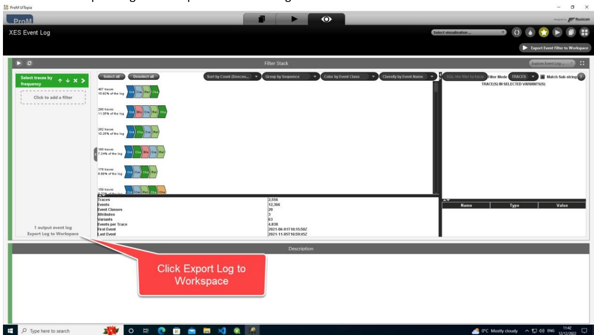
Figure 20 - Image showing how to export the filtered event log to the ProM workspace
