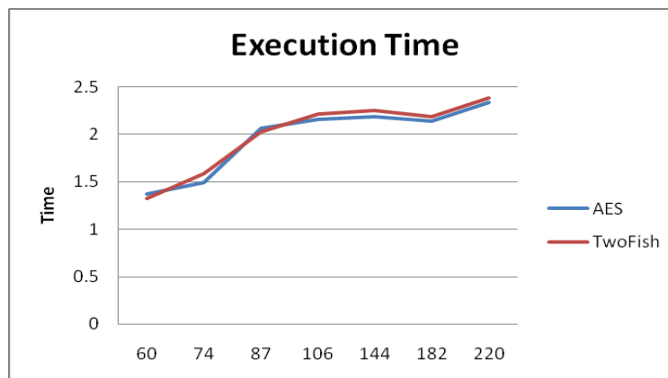
Figure (10): Execution time of algorithms with respect to the size of the password
