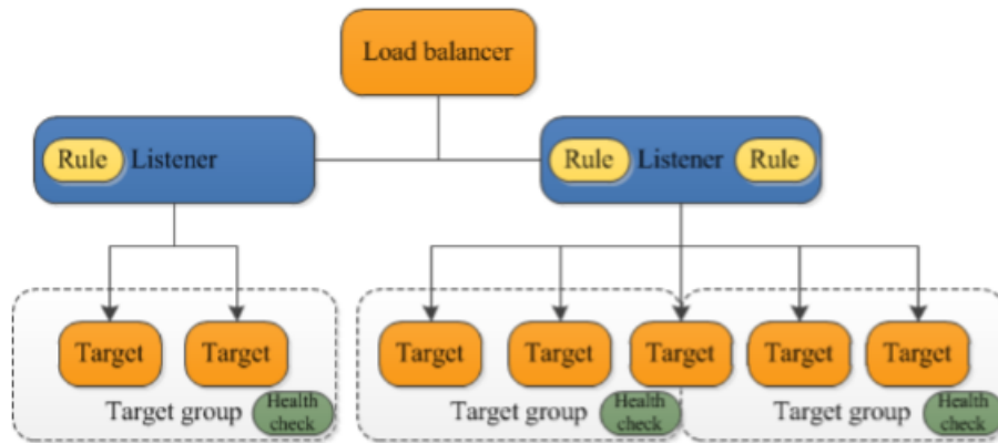
Figure 7. Shows a High-Level block diagram of a Load Balancer
