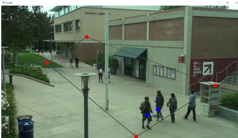
Figure 9: Mouse points selection to convert the frame into Bird-eye view
