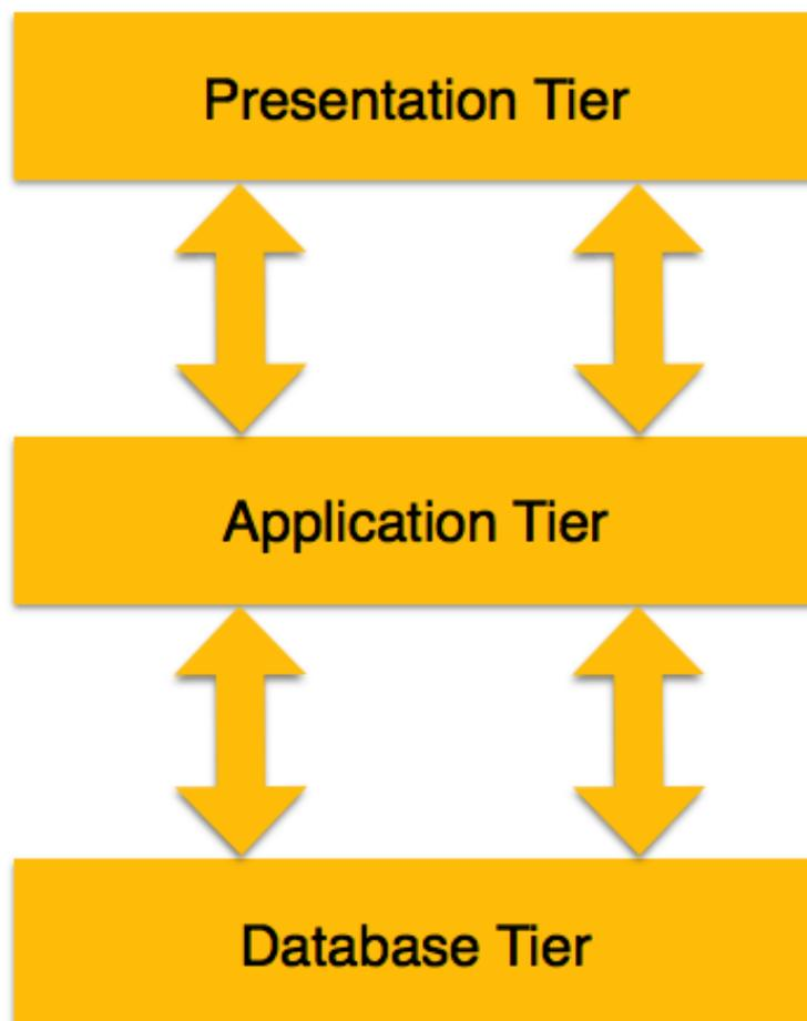
Figure 12: Three Tier Architecture
