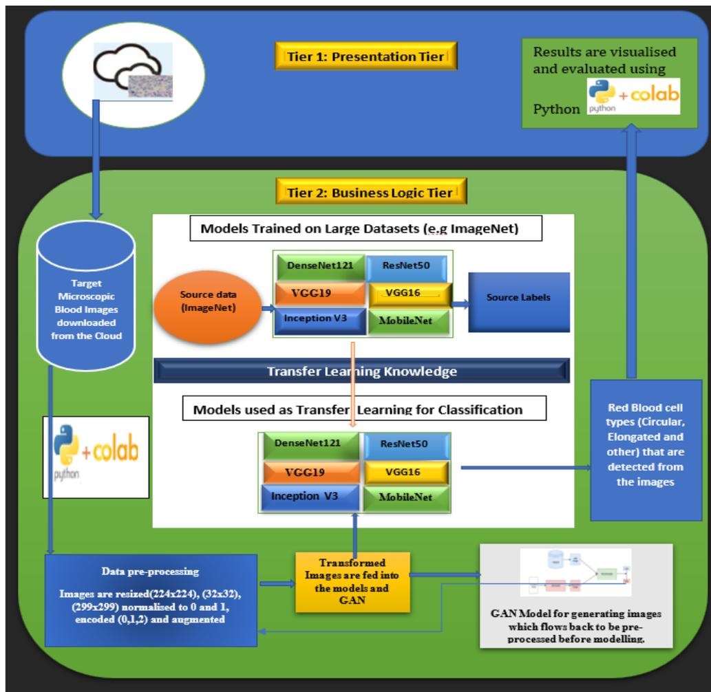
Figure 4: Design process for Sickle Cell Anemia Classification
