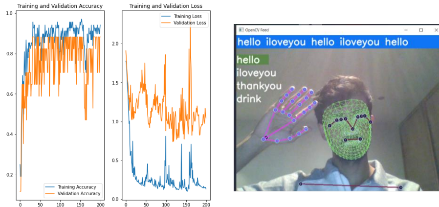
Figure 9: GRU Model Evaluation and Accuracy/Loss graphs
