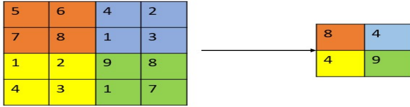
Figure 8: Max Pooling Operation with filter 2*2 and stride 2
