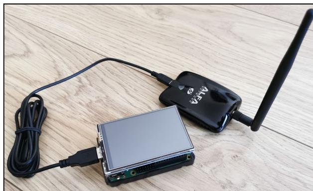
**Figure 1:** Portable attacking machine Raspberry Pi with Alfa AWUS036NHA
