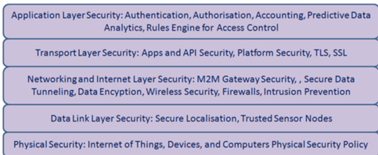
Figure 2: A multi-layered security architecture of CPS/IIoT for the modern computing paradigm of Industrial Control Systems.
