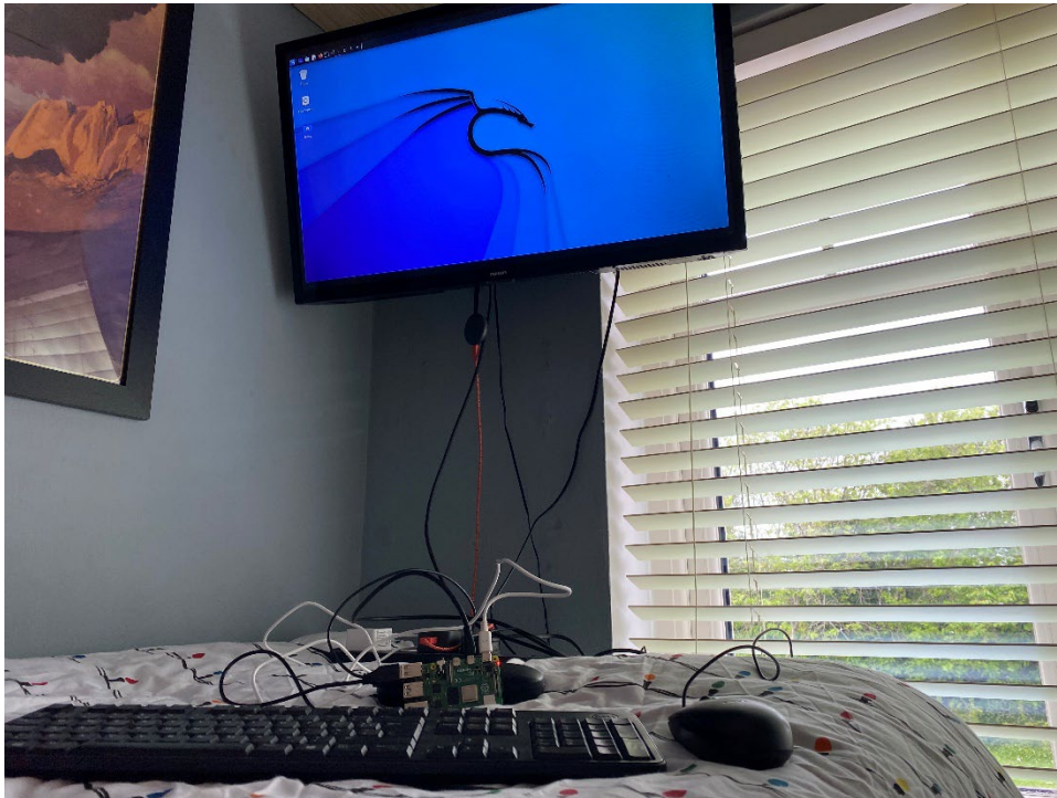
Image 4 – Raspberry Pi set up with all components running Kali Linux
