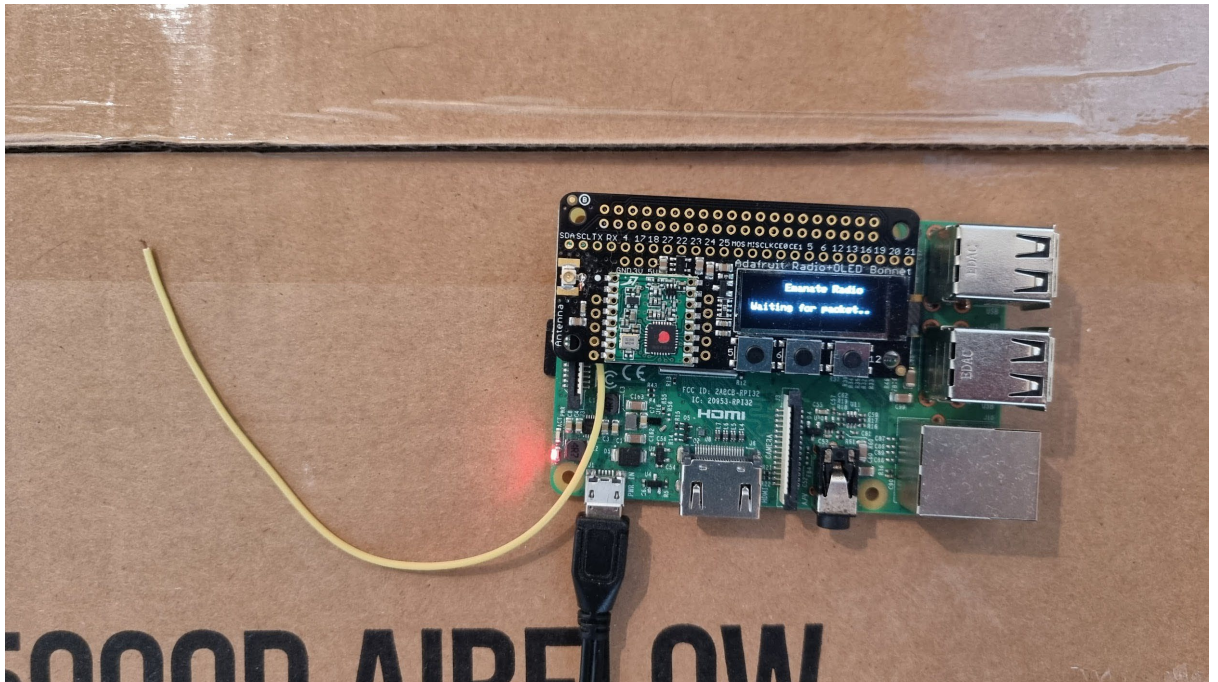
Figure 2.4.1.1: RFM69 Radio Bonnet and Raspberry Pi
