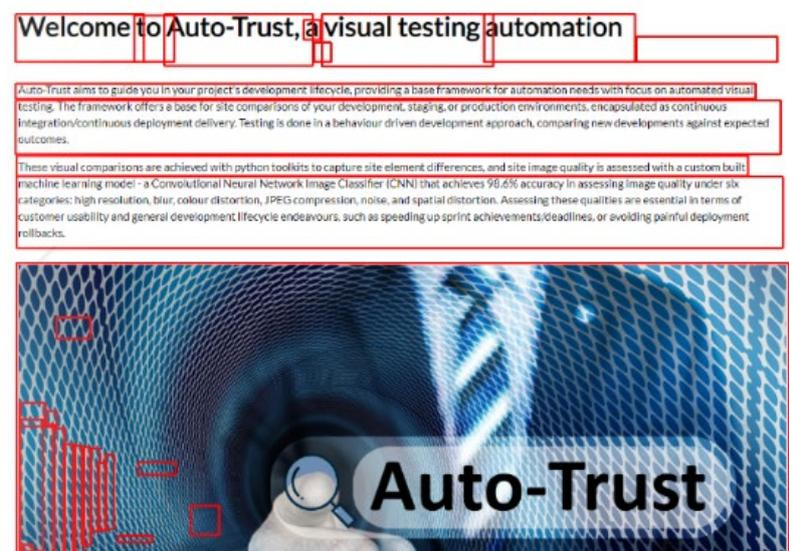
Fig. 60. Consusion in image difference assesement between two grayscale, exact images cause by a lareg shift in the page when an element was removed.
