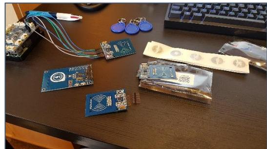
I installed the required libraries on my raspberry pi and began to prepare a script for reading and writing data through RFID. I plugged the first reader in – no result it did not work. Then thankfully the second one worked immediately and I could now read and write data to the tags. For testing, I added 4 variables Food Type, Expiry Date, Calories and Protein content – these would give me a good basis to work off.
