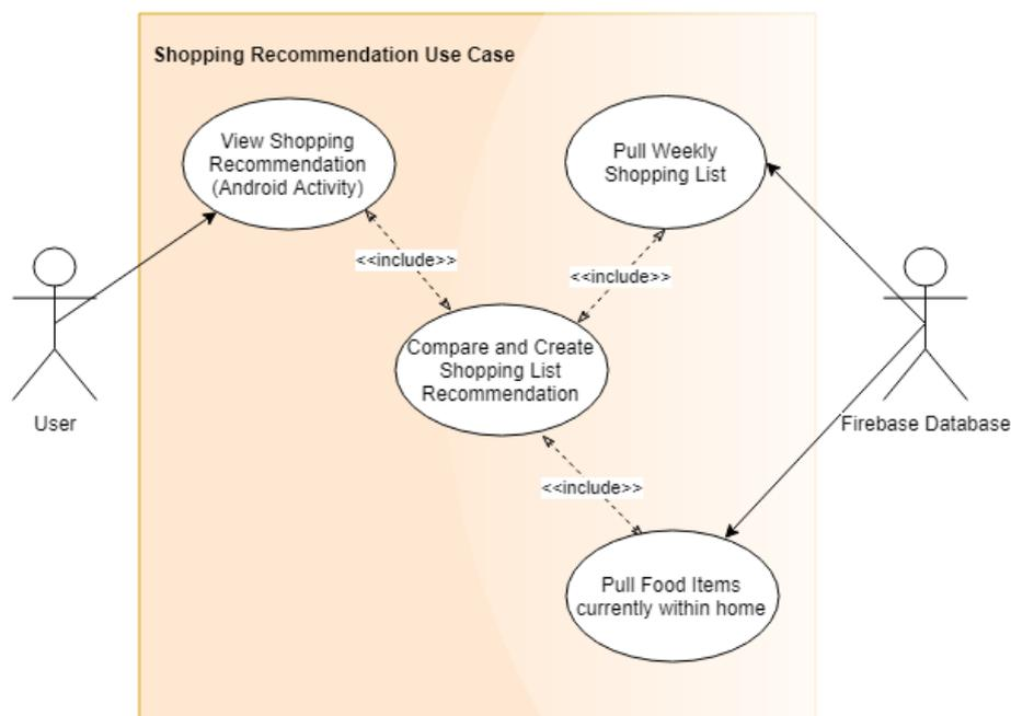
Figure 21 - Requirement 11 Use Case Diagram
