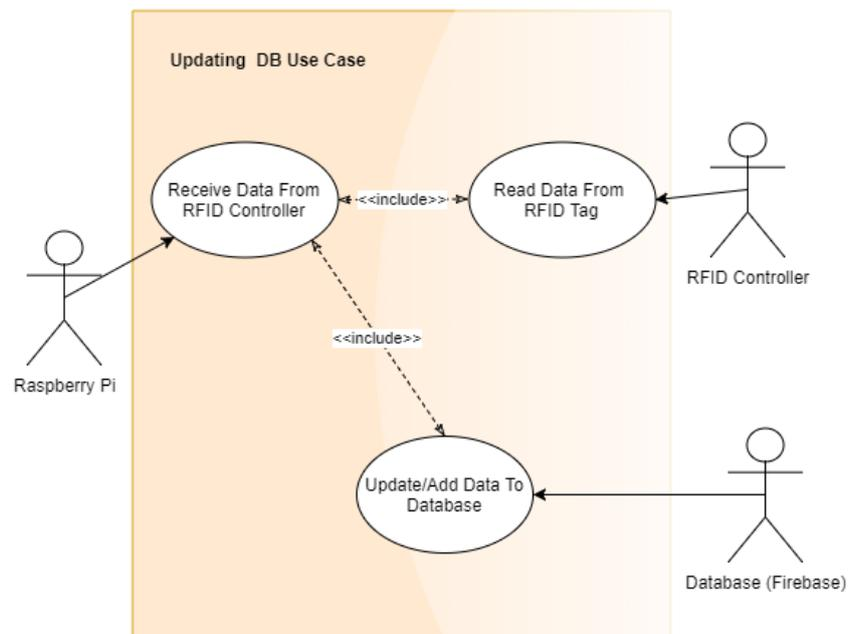
Figure 13 - Requirement 3 Use Case Diagram
