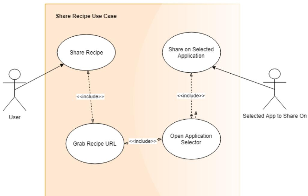
Figure 18 - Requirement 8 Use Case Diagram
