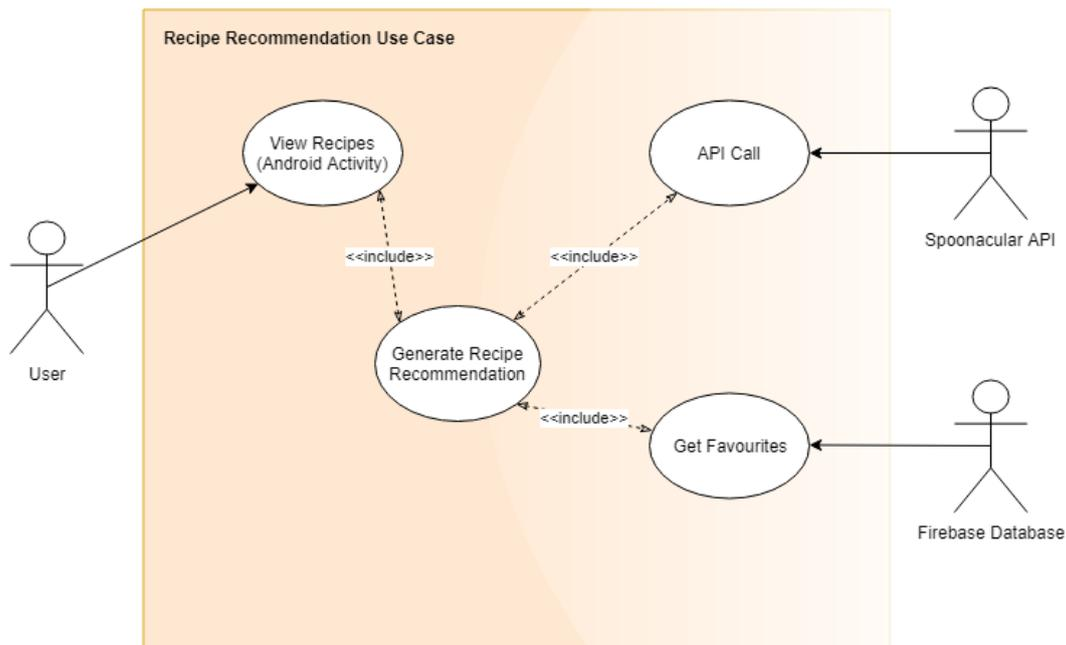
Figure 20 - Requirement 10 Use Case Diagram
