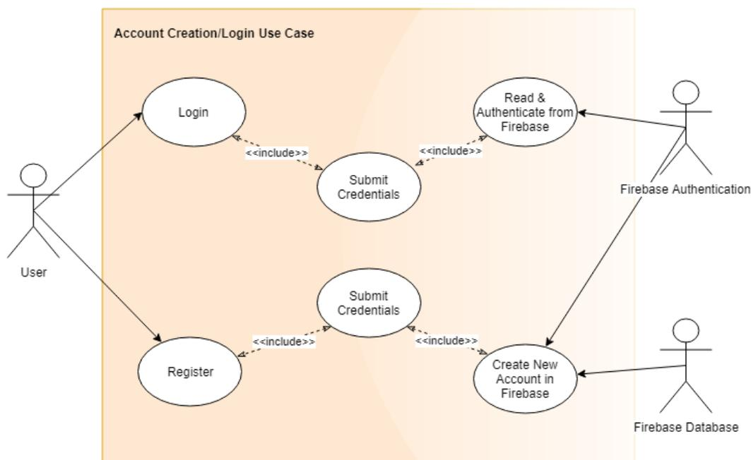
Figure 11 - Requirement 1 Use Case Diagram
