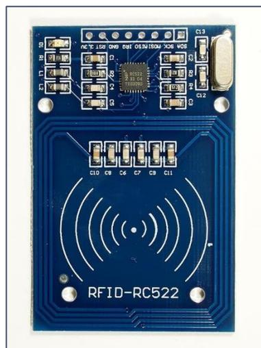
Figure 90 - RC522 RFID Controller
