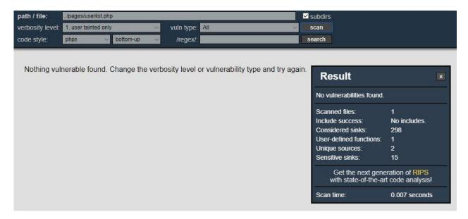
All files that are responsible for any type of php functionality in the website are secured from any input from an user, no vulnerabilities were found in the files that users could use. The tester is only complaining on code sinks for doing things like:
