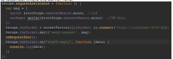
Then I am sending the created message to the server using socket.io. The message passes as a parameter the Object. After sending the socket message, the onRequestSent() message is sent which updates the client's screen view by disabling the "Request Assistance" button and displays next to it the "Cancel Request" button.
