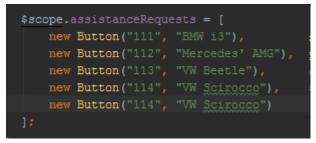
As you can see, when a client taps on button to require assistance, a message with the car's beacon id and car's name is sent to the server which in turn is forwarded to the staff's front-end app and stored in the assistanceRequests list.
