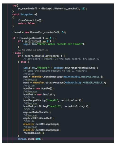
After reading call closeConnection(); (switches device into off state)
