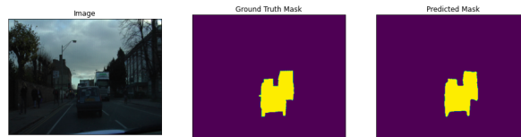
Figure 16: Segmented mask result of class car for FPN-ResneXt-50
