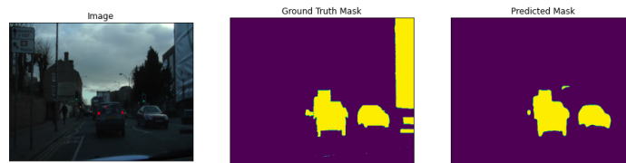
Figure 10: Segmented mask result for U-Net-ResNet-50
