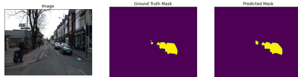
Figure 15: Segmented mask result of class car for FPN-ResNeXt-50
