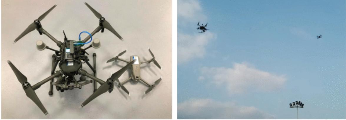
**Figure 4:** A DJI M210 with XT2 camera used to capture target micro-UAV (DJI Mavic). Image referred from (Zheng et al.; 2021)
