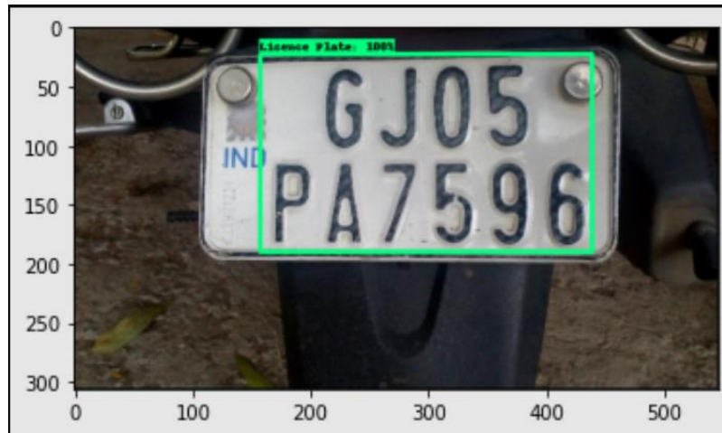
Figure 7: License plate detection using MobileNetV2 FPN lite
