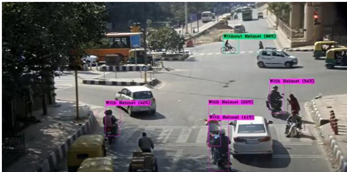
Figure 5: Helmet detection snapshot from video using YoloV4-Darknet
