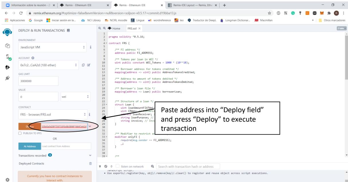
Deploy contract and check menu option made up of 2 orange buttons called "non-payable functions" which are used to input parameters and create a transaction. There are 5 blue buttons called "constant functions" which will only return values when clicked.
