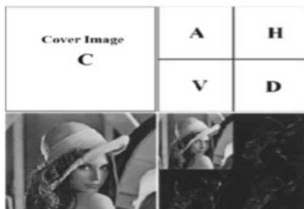
Fig 1. Decomposition using Haar Discrete Wavelet Transform [8]
