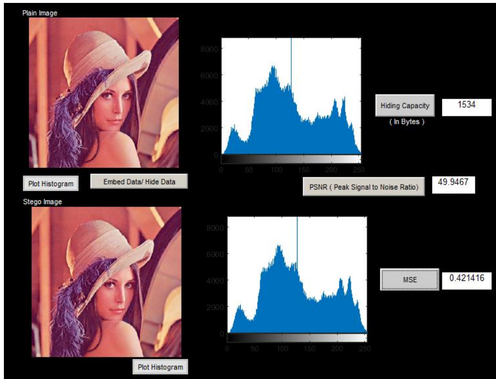
Fig 10. Represents the embedding of the ciphertext in the plain image. Once the ciphertext is embedded in the plain image, it is converted into a stego image. In order to calculate the quality parameters of the stego image here, the Peak Signal to Noise Ratio (PSNR) and Mean-Square Error (MSE) value is calculated.
