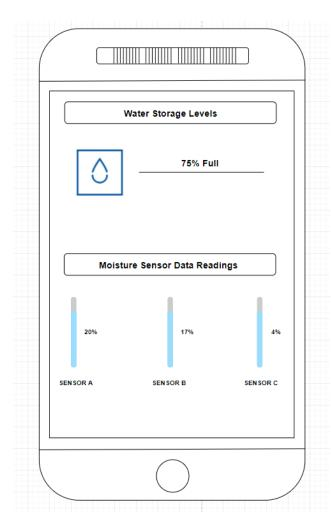
The mobile application is mainly going to be a display unit. The UI for the mobile app should clearly show the number of sensors you have installed in the system and the ultrasonic ranger data should show the amount of water that is left in the storage tank.
