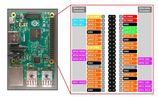
The GPIO pin layout was extremely important as I need to know which pins corresponded to each part of the board
