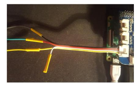
After the modifications were made to the cables, the moisture sensors could be plugged directly into the GrovePi analog ports. The three wires now returned analog reads with values measuring from 0 to 1023. These values could then be converted into percentages using some simple maths and displayed on the application.
