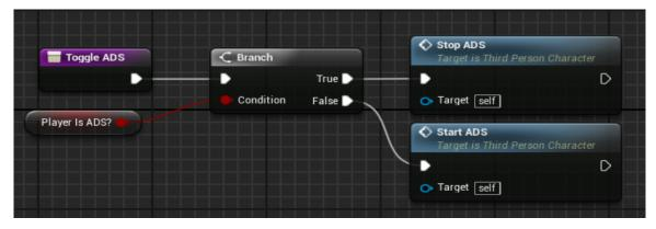
In StartADS and StopADS we can see how the characters movement and orientation is set to be different during each being set as true.
