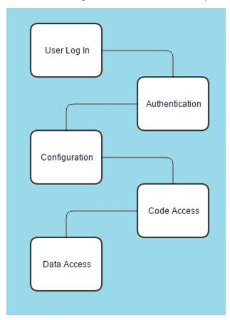
The user must enter their log in credentials, which are sent to the database for a validation check. Once confirmed a connection is opened and the data can be accessed.
